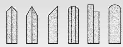
Special Edge Shape (by Grinding)
